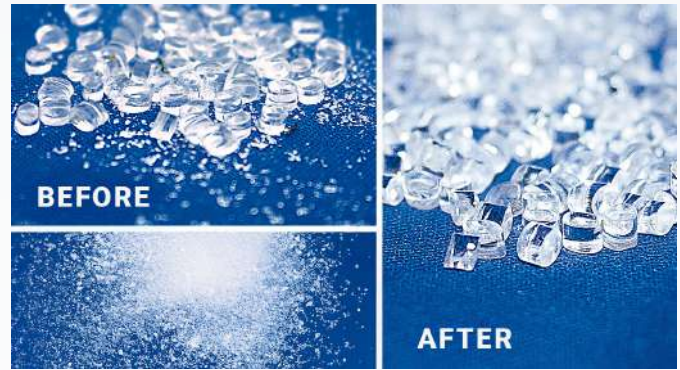
Example: PMMA raw granulate before and after dedusting.
