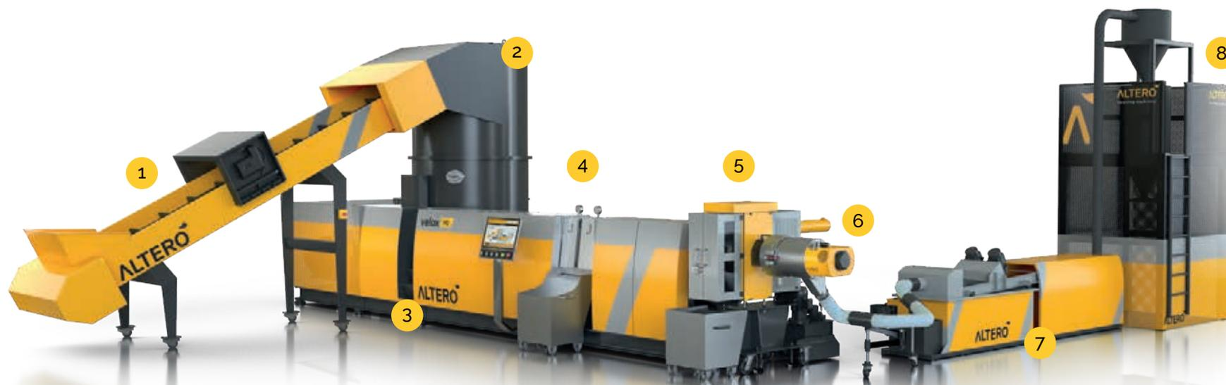
1 **Feeding belt** with metal detector to work with film or materials with very low bulk density.
