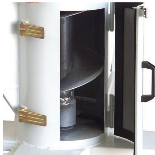
Detail of the inspection door of the mixing screw.
