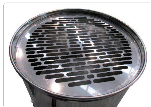
Metal grid to support bag during emptying
