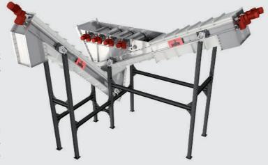
As a rule, a friction washer is placed downstream from the separation tank, because this allows for separation of large quantities of liquids from the material.
